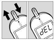
**5** If you do not want to store the test result in the memory, pull out the Test Strip and *quickly* insert it back into the Meter (within 2 seconds).
